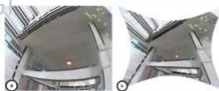
Figure 1: Edges corresponding to straight lines in the real world are detected (a) and the plumblne constraint is used to compute the distortion parameters, giving the rectified image (b)
