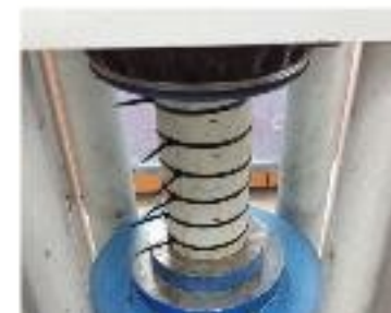
a Polyamide tie reinforcing, b load ring test of partially activated film and c, d load ring test of diametrically ended film
