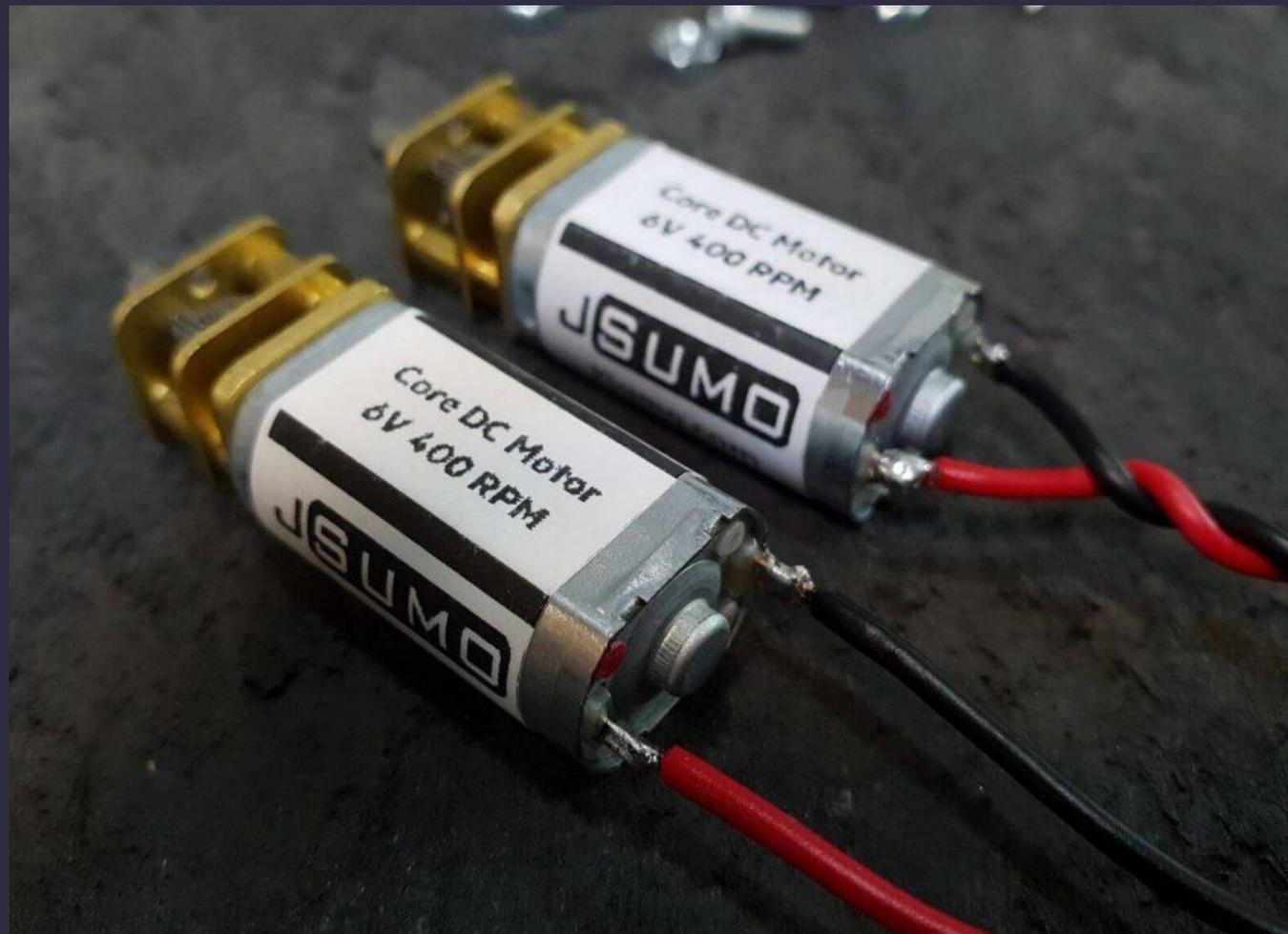
Solder motor DC connections
